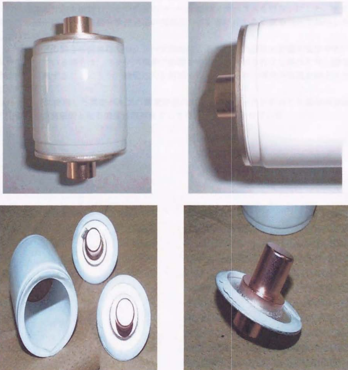
Fig.6-29 Photograph of joint crack for a vacuum interrupter
