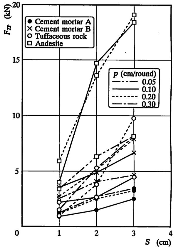
Fig.3 Relationship between peak normal force  $F_{ZP}$  and cutting space  $S$  ( $\alpha = \pi/4$  rad)
