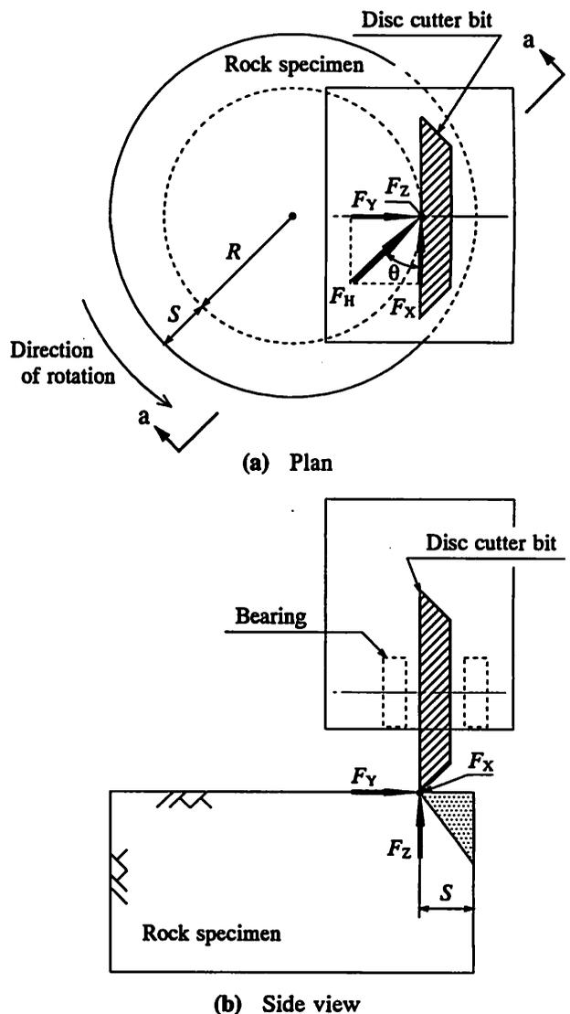
Fig.1 General view of steady state edge excavation
