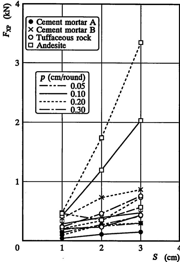
Fig.2 Relationship between peak tangential force  $F_{XP}$  and cutting space  $S$  ( $\alpha = \pi/4$  rad)
