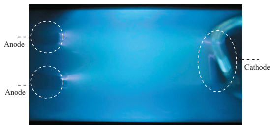
Fig. 3: A photograph of diffuse positive column without external electrode.
