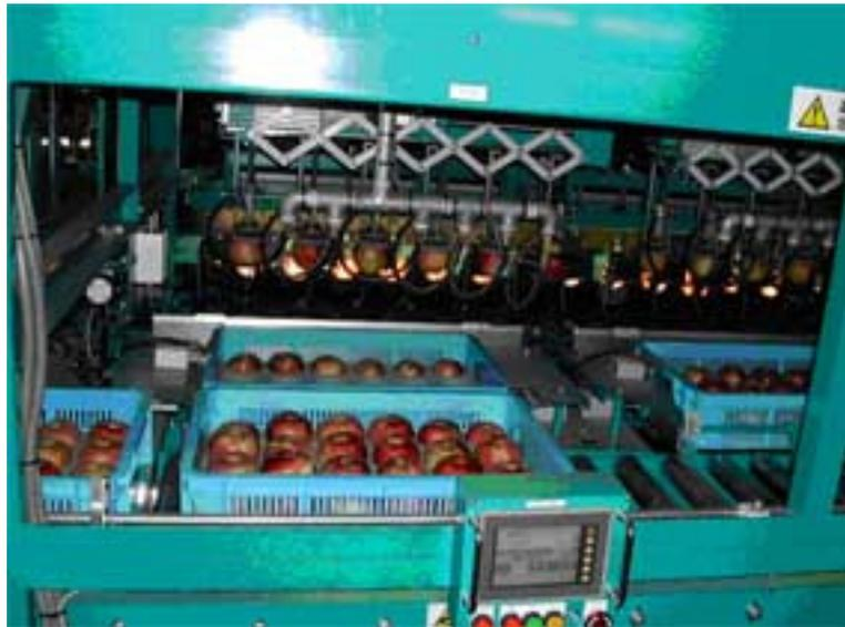
Fig.5 Fruit providing robot and grading robot with containers.
