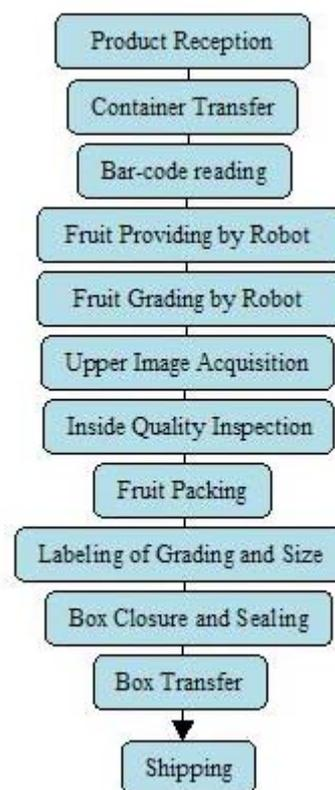
Fig.2 Operation flow of grading system..
