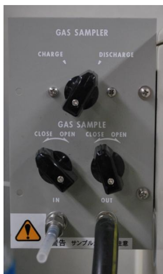
Switch on/off for Input Gas
