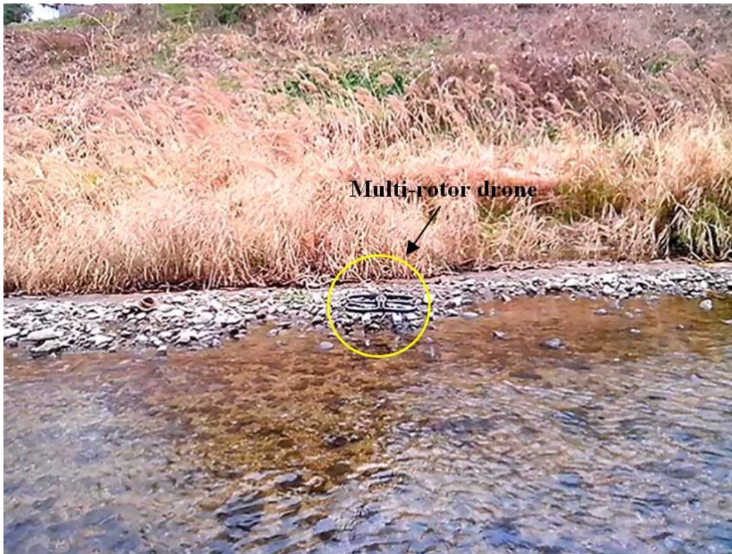
Fig. 3.6 Multi-rotor drone on the start position at the riverside in a flying experiment to perform a manual flight with off-line image processing
