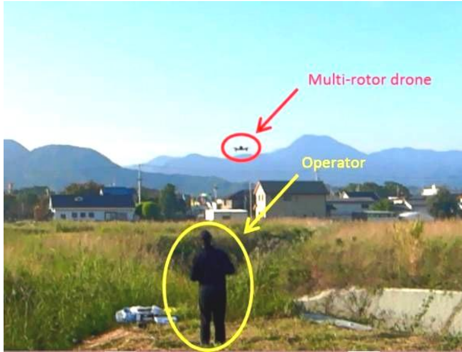
Fig. 4.4 Scene in which static photo images and videos images of the environment around the river were captured by the fisheye-lens camera installed on the Parrot Bebop Drone flight-controlled manually
