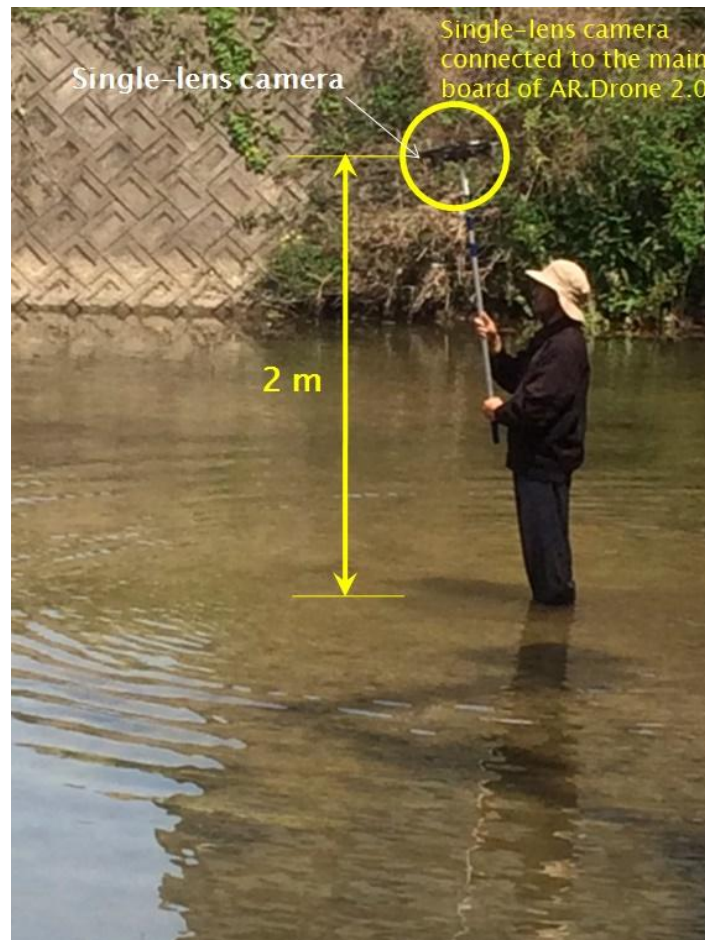
Fig. 2.12 Single-lens camera connected to the main board of AR.Drone 2.0 attached to a stick held by a person in the center of a river in an experiment to capture photo images of river scenes
