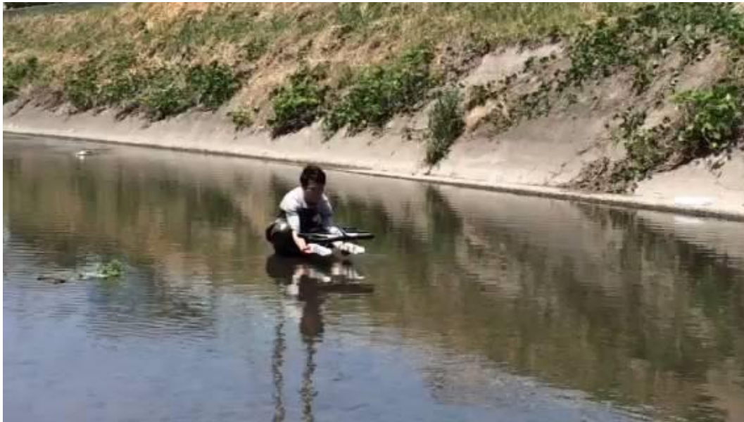
Fig. 3.20 Multi-rotor drone holded by a person in the center of river to perform an autonomous flight in an experiment carried out on the curved river with a large slope
