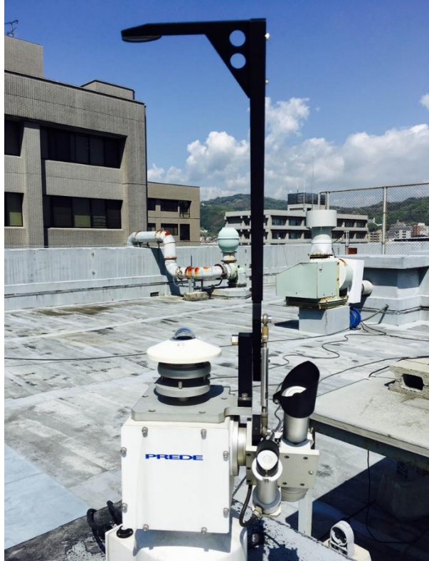
Figure 4.6: Combination of a pyranometer (Kipp & Zonen, CMP-3), sunlight shielding device and solar tracking device to measure the direct beam and diffuse solar radiation
