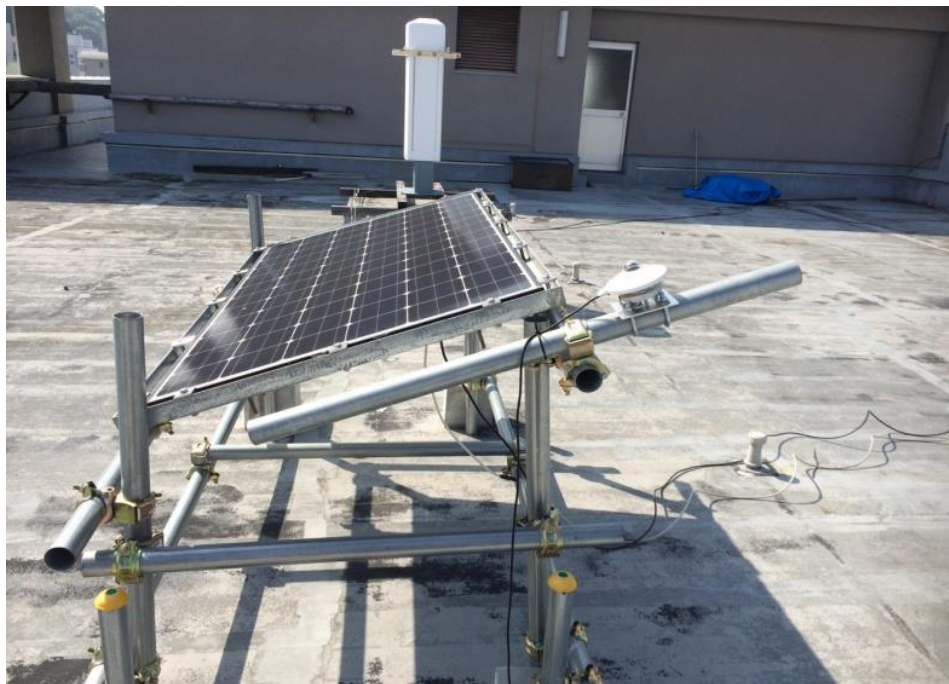
Figure 4.5: Pyranometer (Kipp & Zonen, CMP-3) installed along with the tilted solar panel
