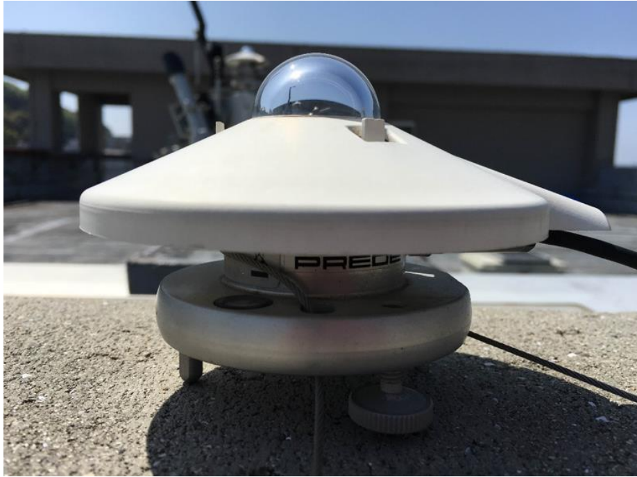
Figure 3.2: The pyranometer (CMP-3EU, Kipp and Zonen) installed at Ehime University
