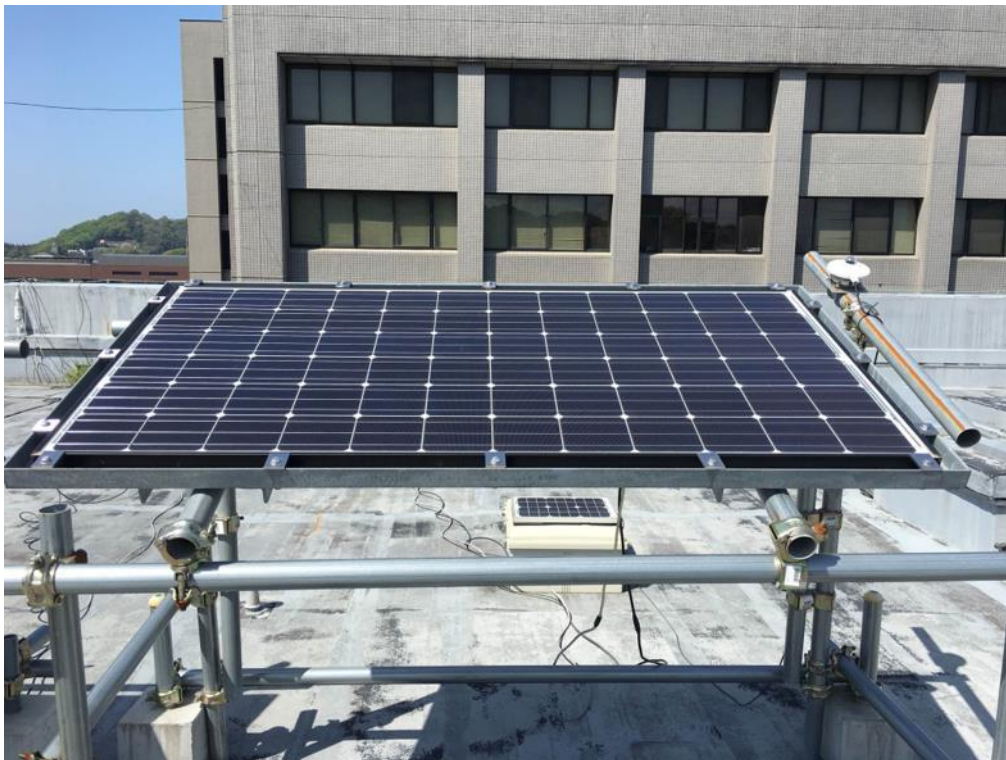
Figure 4.3: Solar panel installed at a tilt angle of 20^\circ due south
