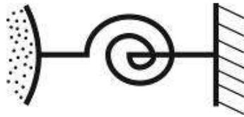
Fig. 2.7 Boundary modeled with rotational spring elements
