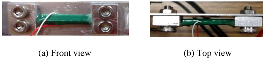
Fig.3.3 Piezoelectric actuator with clamped mechanism
