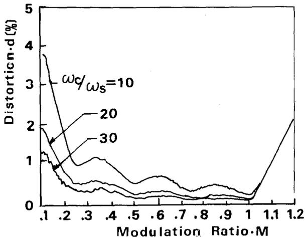
Fig. 12 Distortion of PWM inverters waveform (2-step switched modulation type,  $N=4$ ).
