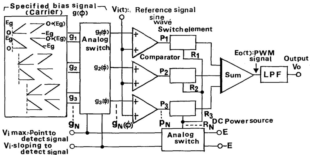
Fig. 3 Basic circuit construction of 2-step switched modulation type multilevel PWM sinusoidal inverter.
