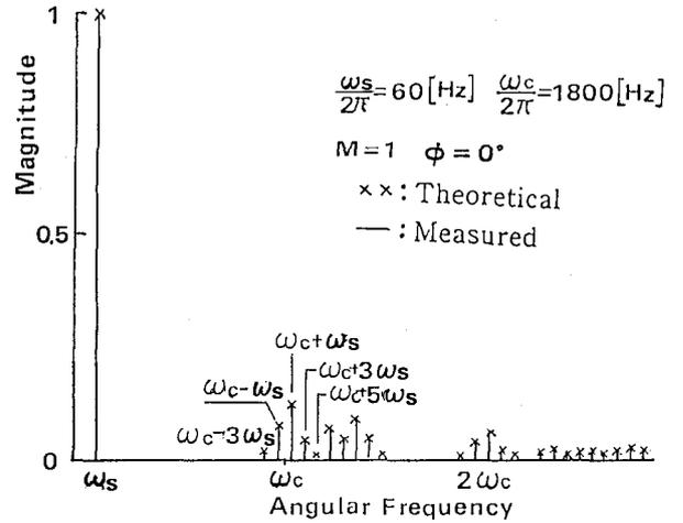
Fig. 9 Compound PWM frequency spectrum.
