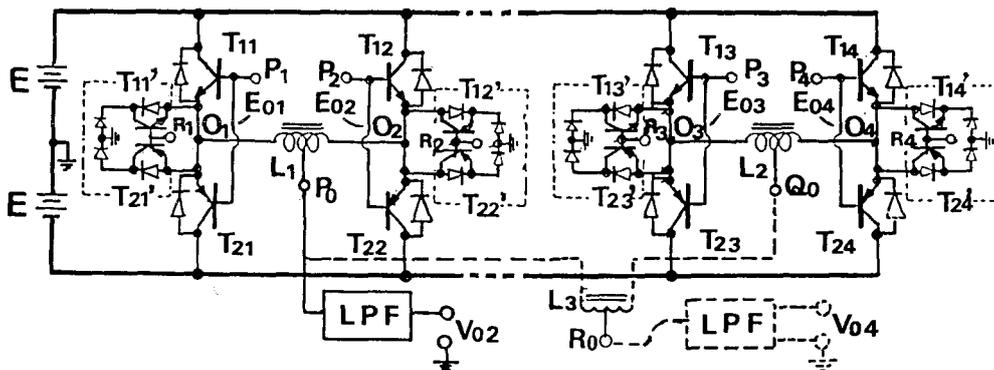
Fig. 13 Circuit configuration of main multilevel inverter (2-step switched modulation type).
