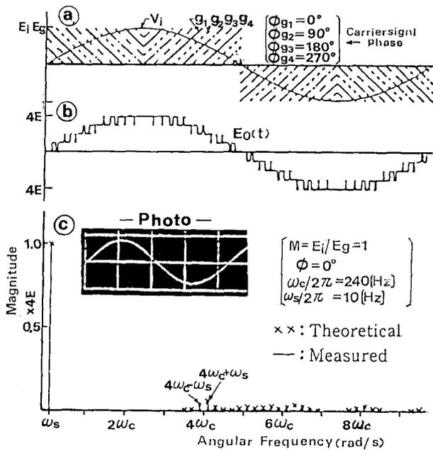
Fig. 6 2-step switched modulation type multilevel *PWM* inverter operation and its frequency spectrum ( $N=4$ ).
