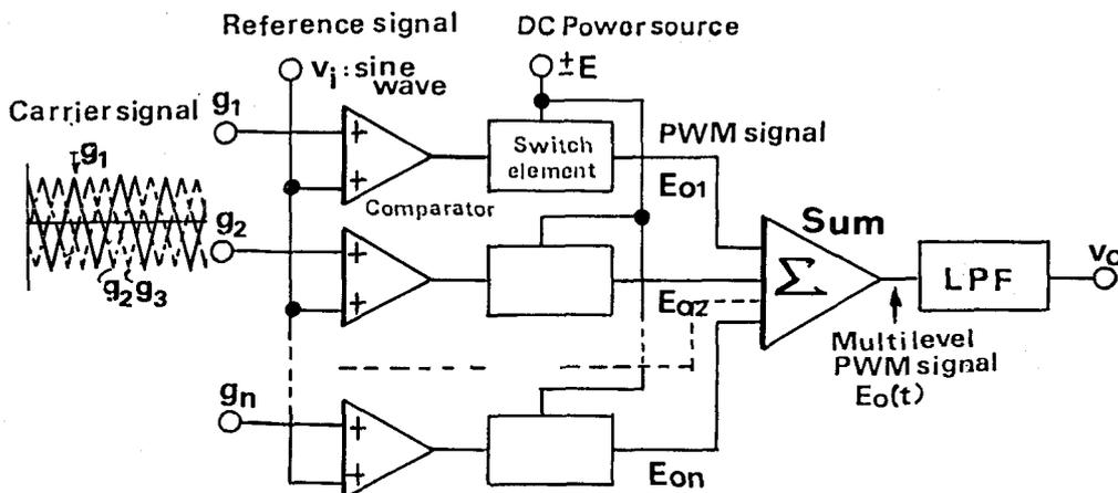
Fig. 1 Basic configuration of multilevel *PWM* sinusoidal inverter.
