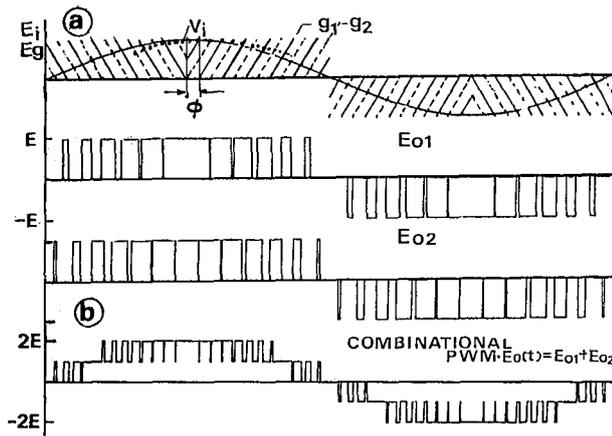
Fig. 2 Operation principle of 2-step switched modulation type multilevel PWM ( $N=2$ ).
