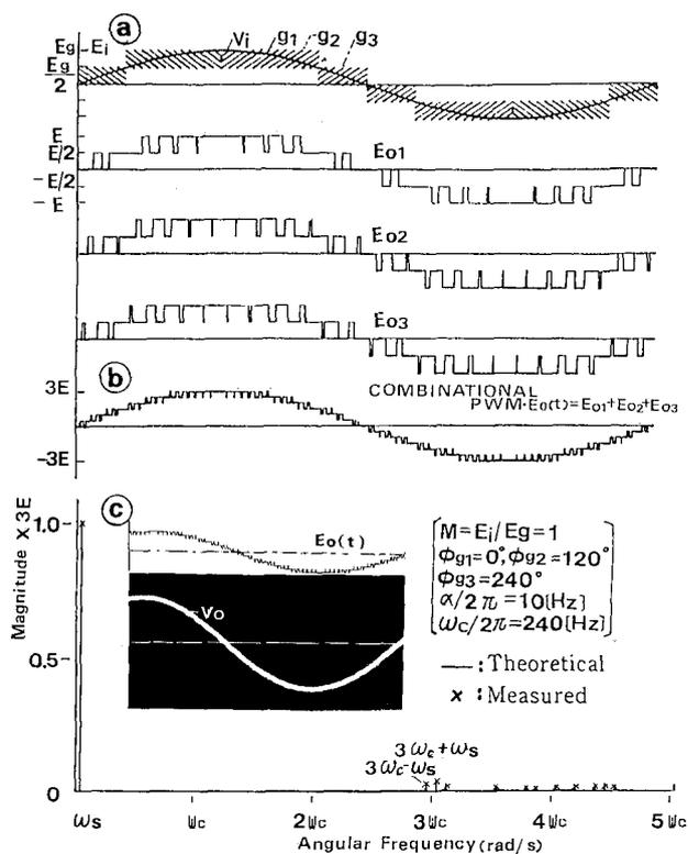
Fig. 11 Compound modulation type multilevel PWM sinusoidal inverter operation and its frequency spectrum ( $N=3$ ).
