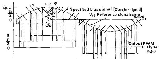
Fig. 7 Operation principles of compound *PWM* sinusoidal inverter.
