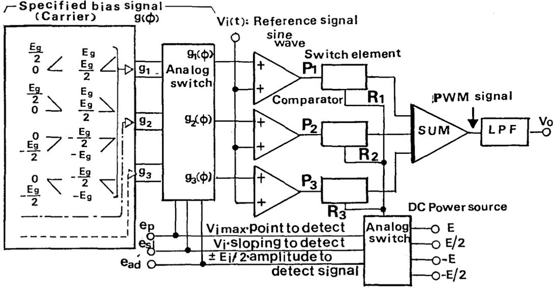
Fig. 8 Basic circuit construction of compound modulation type multilevel PWM sinusoidal inverter (N=3).
