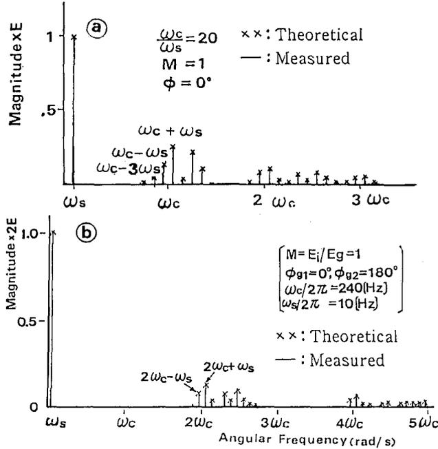
Fig. 4 (a) : 2-step switched PWM frequency spectrum.
