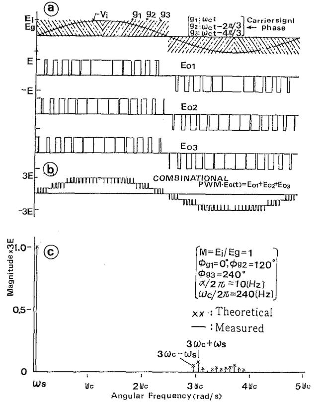
Fig. 5 2-step switched modulation type multilevel PWM operation and its frequency spectrum (N=3).
