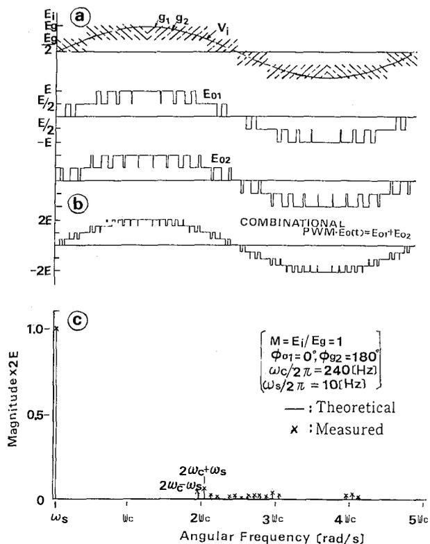
Fig. 10 Compound modulation type multilevel PWM operation and its frequency spectrum ( $N=2$ ).
