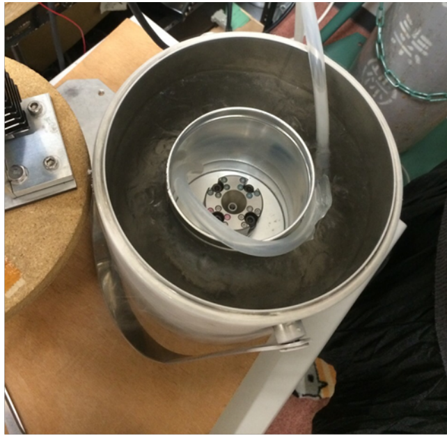
Fig.12 A loading system for liquid Ar into the DAC under low temperature.
