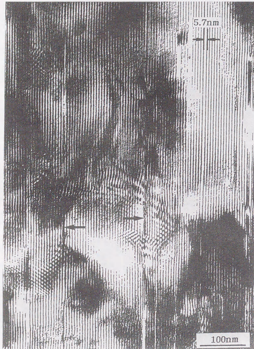
Fig.6・9 Transmission electron micrograph showing (0001)_{\delta} lattice image.
